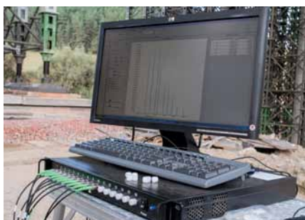
Figure 2: Automated monitoring system – Interrogator FBG Scan 816
