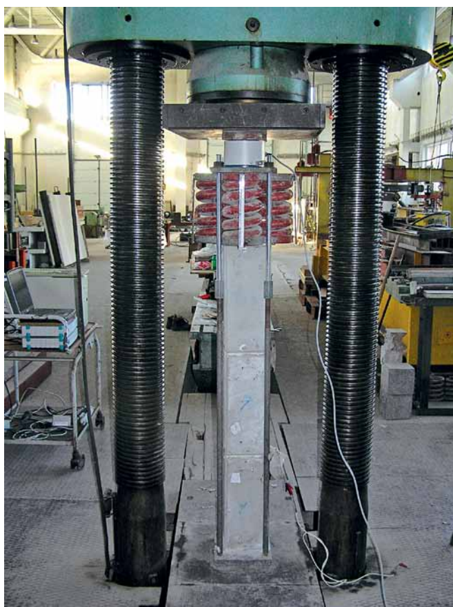
Obr. 3 Zostava na meranie dotvarovania betónu Fig. 3 Set-up for measuring creep
