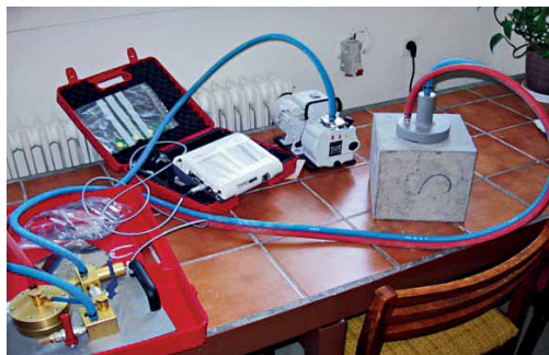
Obr. 1 Súprava Torrent Permeability Tester Fig. 1 Set of the Torrent Permeability Tester device
