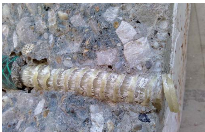
Obr. 3 Schéma usporiadania pull-out skúšky a vzorky po porušení Fig. 3 Arrangement of the pull-out test and specimens after failure
